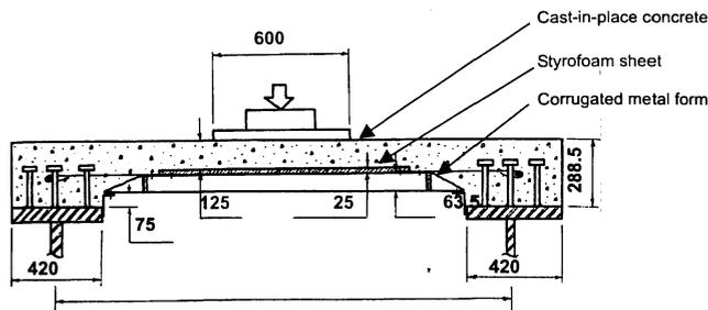
Fig. 6. Precast concrete stay-in-place formwork with cast-in-place concrete.
