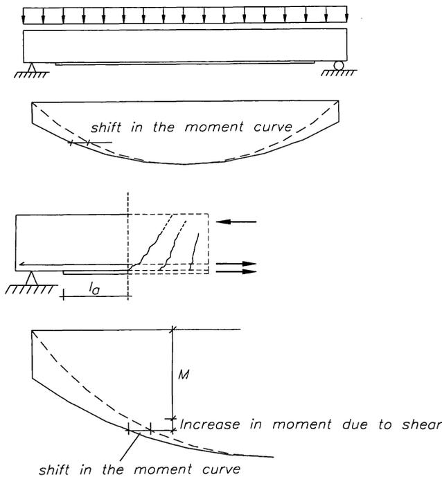
avoid a possible failure by delamination of the FRP initiating at intermediate cracks (Täljsten 2002; Teng et al. 2002).
