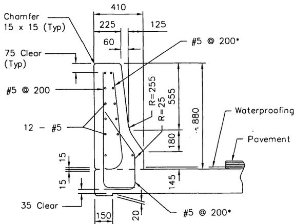
**Fig. 8.** PL-2 barrier wall with GFRP bars (dimensions in millimetres).
